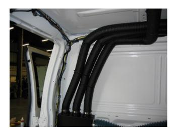
Route hose straight up from the HVAC unit and tie tight to corner of the van
